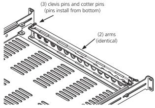
Figure 5. Attaching the cable arms.
